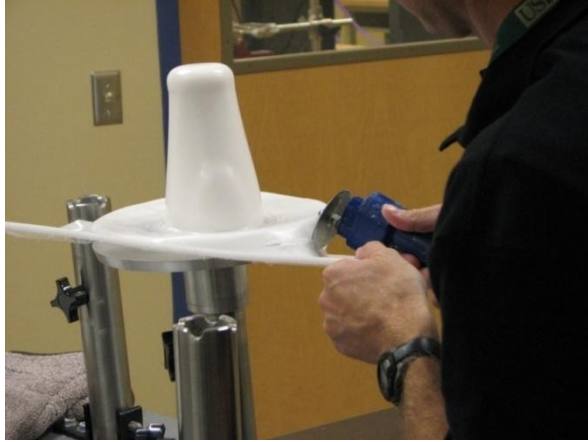
Figure 35: Preliminary thermoformed socket using 3-D printed mold.
