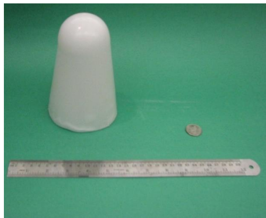
Figure 37: Preliminary thermoformed socket using 3-D printed mold.
