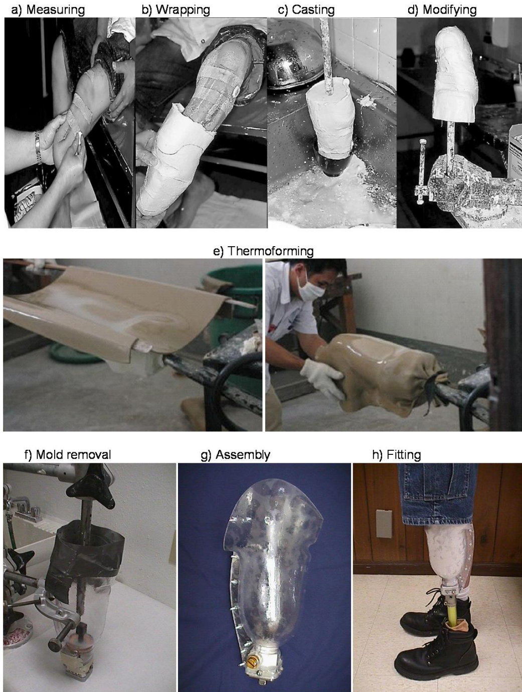
Figure 7: Traditional prosthetic socket manufacturing stages 9, 18, 19 .
