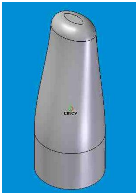
Figure 34: CAD image of the preliminary mold tested.
