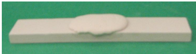
Figure 32: Reinforced specimen for flexural strength test.
