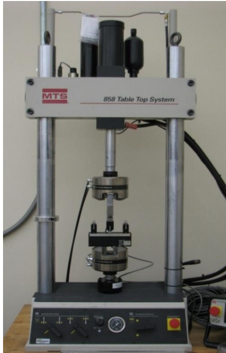
Figure 23: MTS universal testing machine with bending fixtures and low force sensor.
