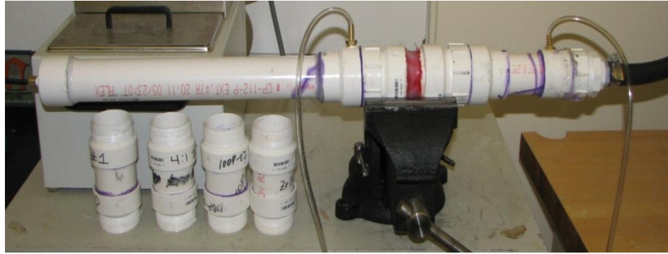
Figure 18: Pneumatic permeability set up.
