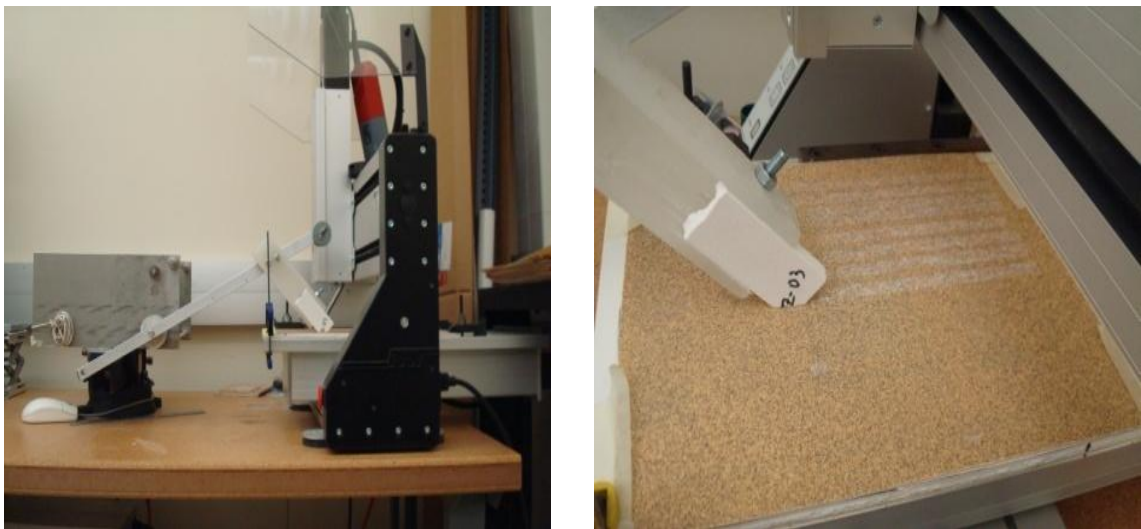
Figure 25: Wear test set up.
